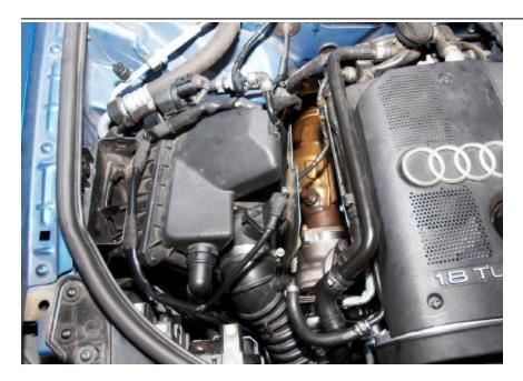
27. Reinstall the top half of air box in reverse order and tighten down two screws and all clamps.
