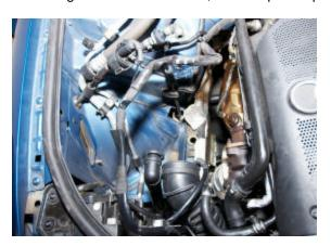
10. Remove bottom of air box from vehicle.
