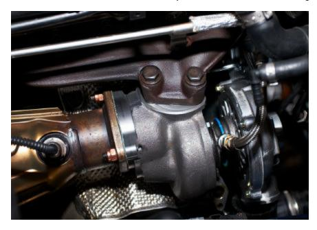
19. Bolt in the new Eliminator turbo by sliding into place. Torque down the turbo to manifold and turbo to catalyst bolts.
