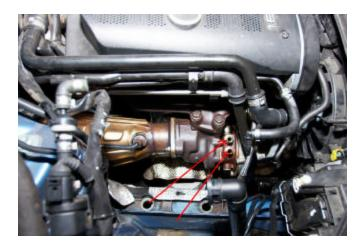
13. Unscrew the oil feed line and coolant feed line from top of turbo.
