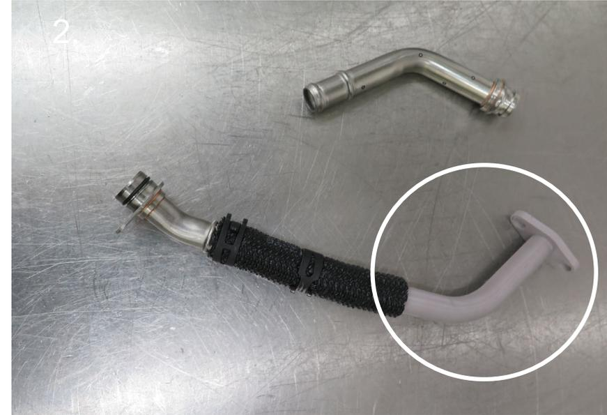
2. Replace with provided oil drain tube
