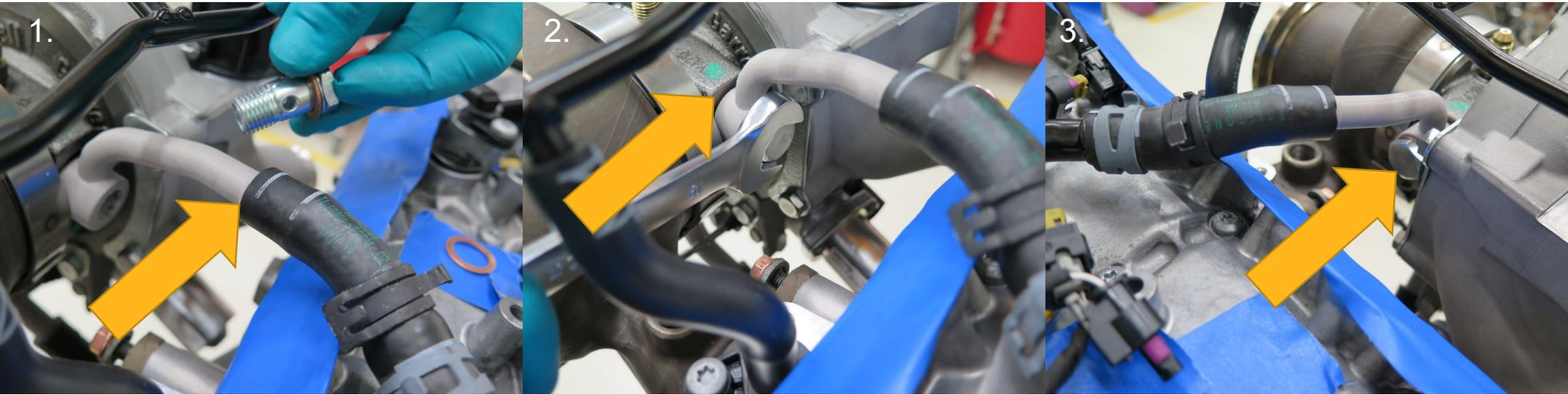
1. Insert water outlet tube into the OEM water return hose. Secure clamp. Place copper washer on the supplied banjo bolt.
