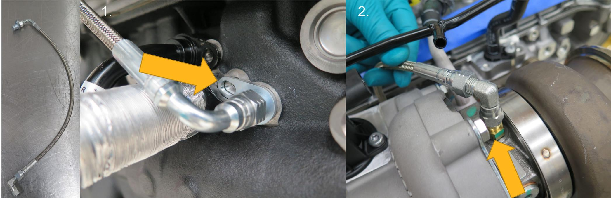
1. Attach oil line to engine using the OEM bolt. Tighten to OE specifications.
