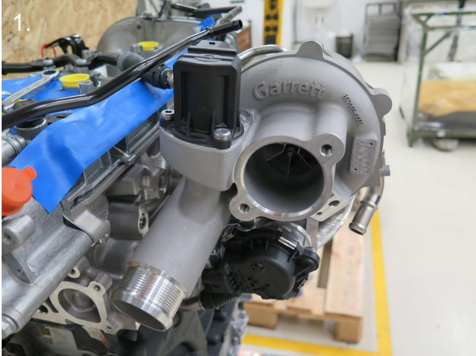
1. Use provided inlet adapter, gasket, and 2 M8 x 20 supplied bolts to attach the compressor inlet
