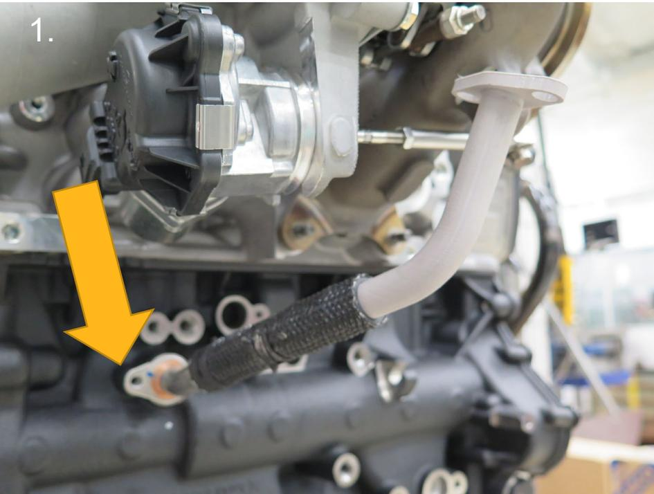
1. Attach to engine block with OE bolt. Tighten to OE specifications.
