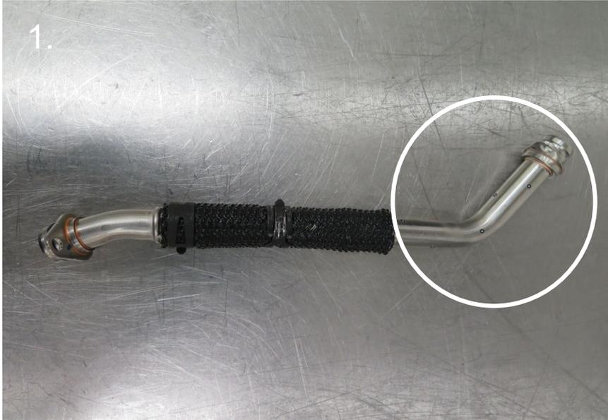
1. Remove the OEM turbo drain tube section
