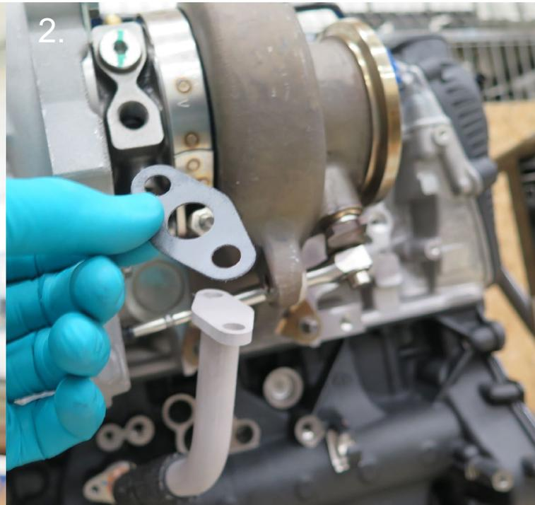
2. Place provided flange gasket on the drain tube flange.
