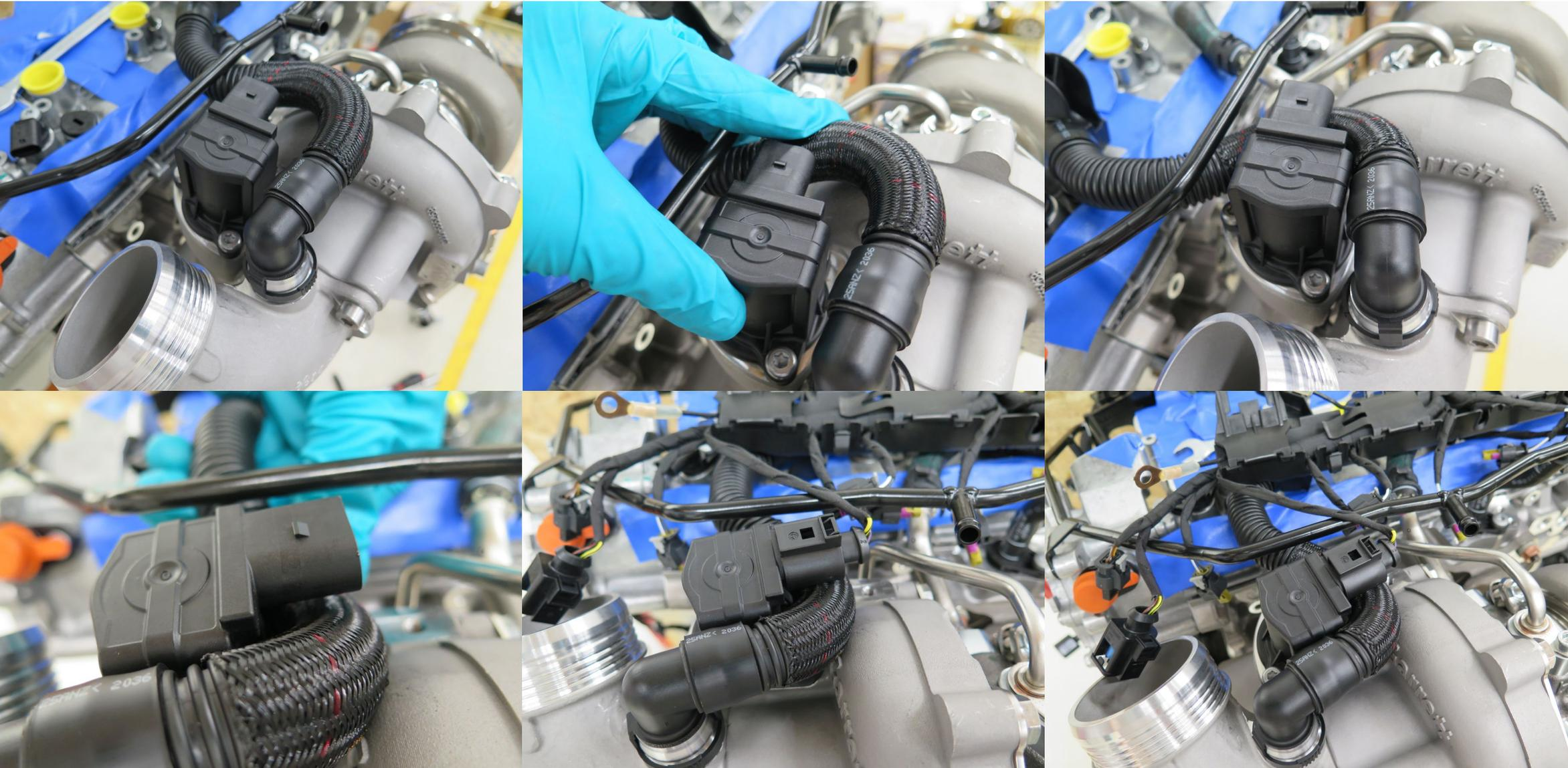
Route crankcase vent hose under electrical connector
