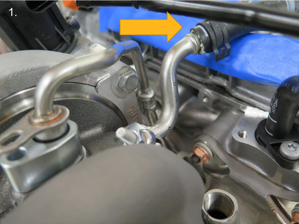
1. Connect water outlet to OE engine hose and tighten clamp
