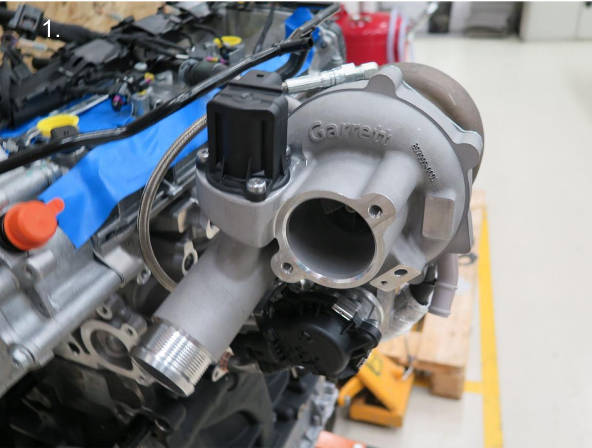
1. Use provided inlet adapter, gasket, and 2 M8 x 20 supplied bolts to attach to the compressor inlet
