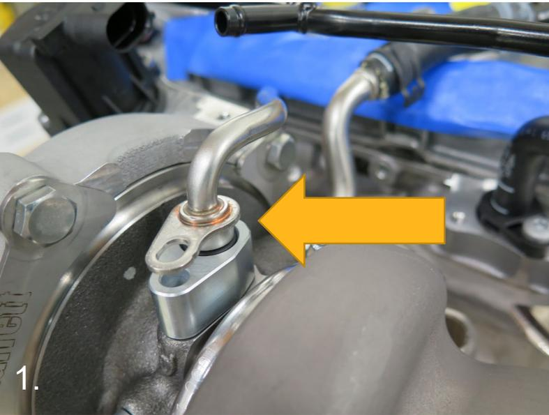
1. Attach OE oil inlet pipe to turbo adapter
