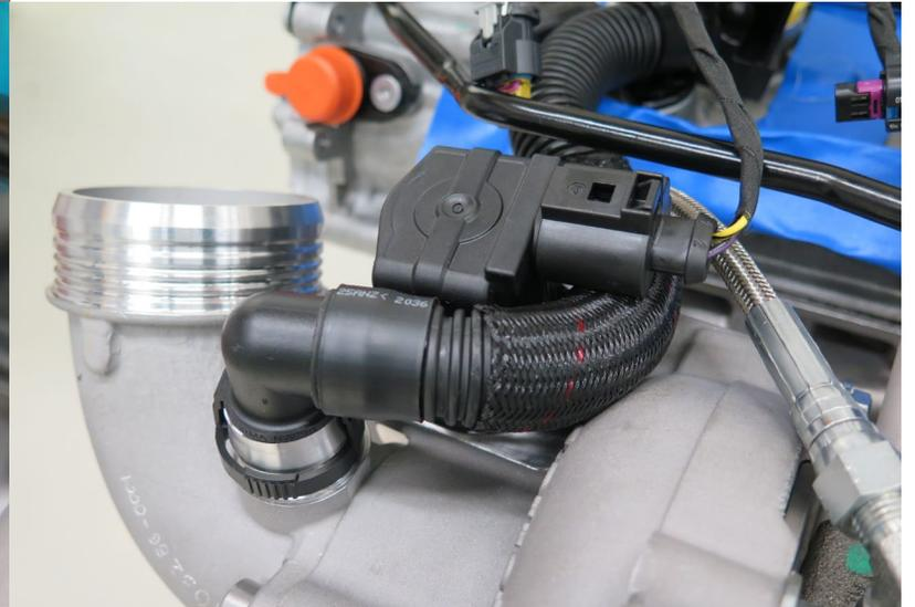
Route crankcase vent hose under electrical connector
