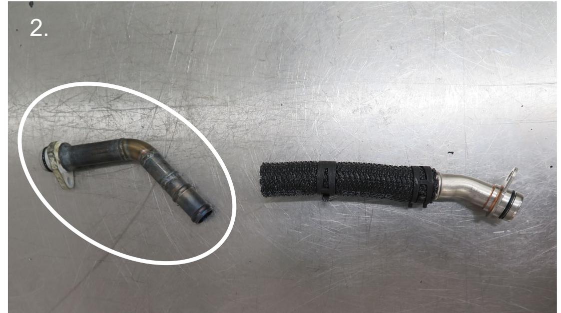
2. Replace with provided pipe and check hose clamp to ensure a tight connection
