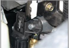
6. Tighten down to 7 ft/lb with 8mm wrench.
