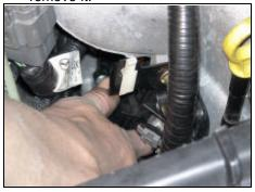
3. Gently pull MAP sensor away from intake manifold (not necessary to disconnect electrical connector attached to it).
