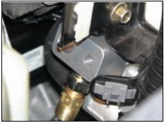
5. Slide MAP sensor into the ATP BCK module and attached to intake manifold with long 5mm bolt and washer provided in the kit.
