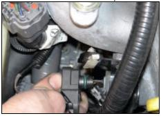
4. Slide ATP BCK module into intake manifold at original MAP sensor location.
