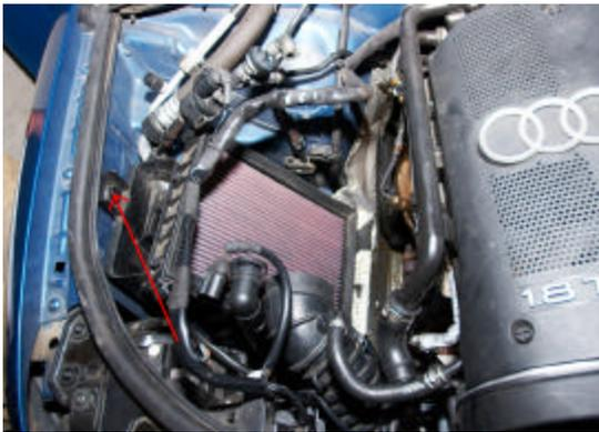
9. Using flathead screwdriver, remove plastic pin holding bottom of air box to vehicle.
