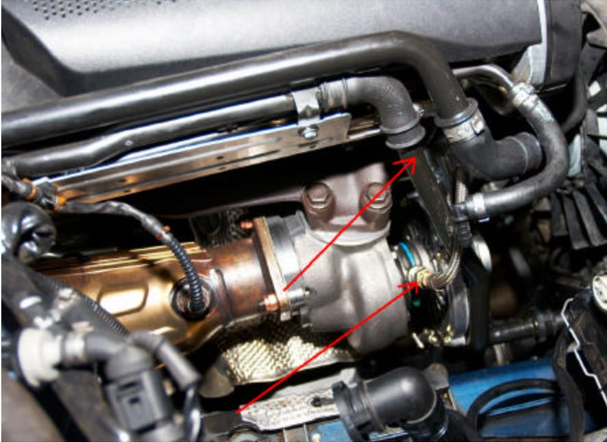
20. Reinstall the oil feed line and the air injection hose. Replace one time use clamp with new clamp provided.
