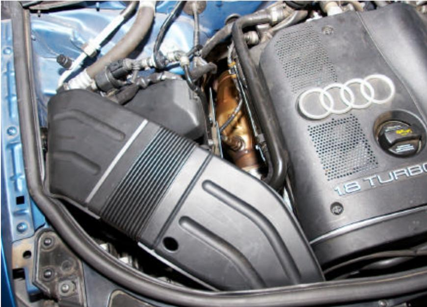
28. Reinstall the top air duct and 2 mounting screws.
