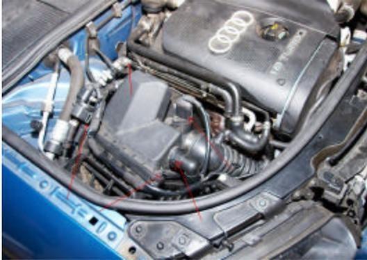
3. Unscrew 2 screws holding air box top to air box bottom.
