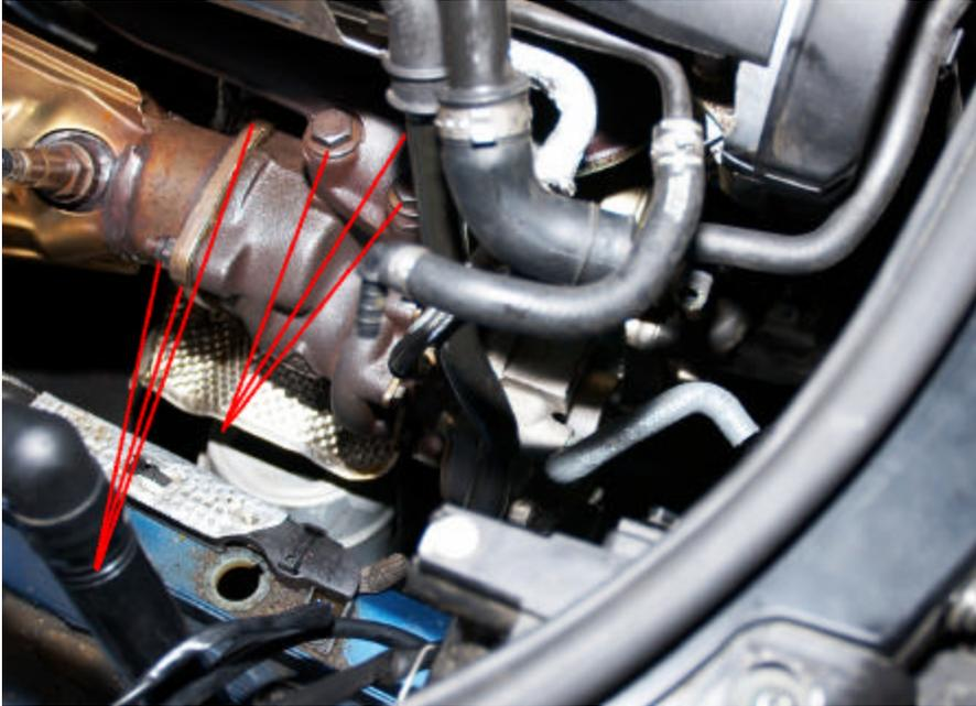
**Installation Tip #2** – Using a spray on penetrating oil (such as liquid wrench lubricant), saturate all the exhaust nuts/bolts (turbo to manifold & turbo to down pipe) and allow it to sit. This will allow any rusted hardware to come loose without breaking. 5 minutes of preparation can save a lot of hours in nut/bolt extracting!
