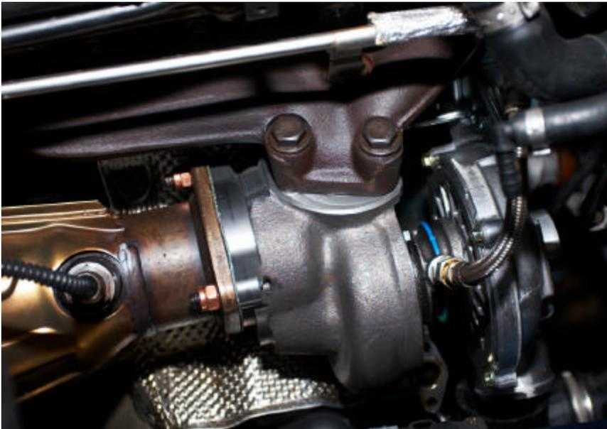
19. Bolt in the new Eliminator turbo by sliding into place. Torque down the turbo to manifold and turbo to catalyst bolts.
