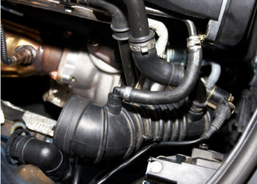
25. Reinstall the stock inlet hose and use clamps provided on all one time use clamps removed.
