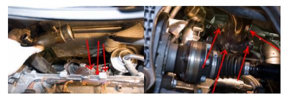
**Installation Tip #2** – Using a spray on penetrating oil (such as liquid wrench lubricant), saturate all the exhaust nuts/bolts (turbo to manifold & turbo to down pipe) and allow it to sit. This will allow any rusted hardware to come loose without breaking. 5 minutes of preparation can save a lot of hours in nut/bolt extracting!
