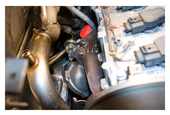
13. Bolt on the new eliminator turbo as shown using new bolts, gaskets, and washers provided.
