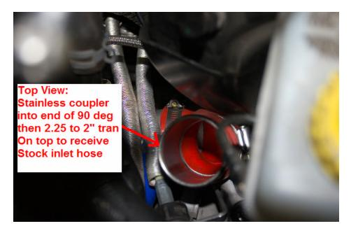
24. With airbox and MAF pipe in original location, run the stock inlet hose into new connection as show:
