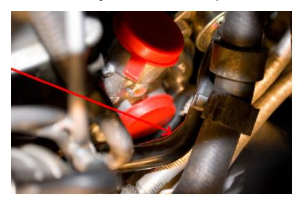
14. Grab black coolant pipe firmly and pull up and bend upwards 1" and towards the compressor outlet nozzle leaving enough clearance only for the outlet hose.
