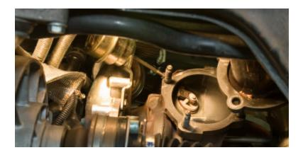
9. Remove the Nuts (17mm) holding downpipe to the turbo.
