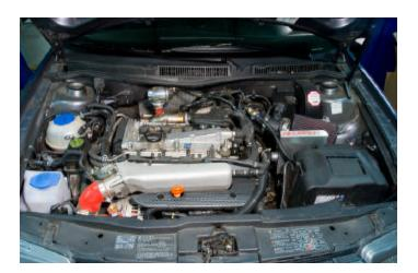
1. Using flathead screwdriver, remove the engine cover from top of valve cover on engine.
