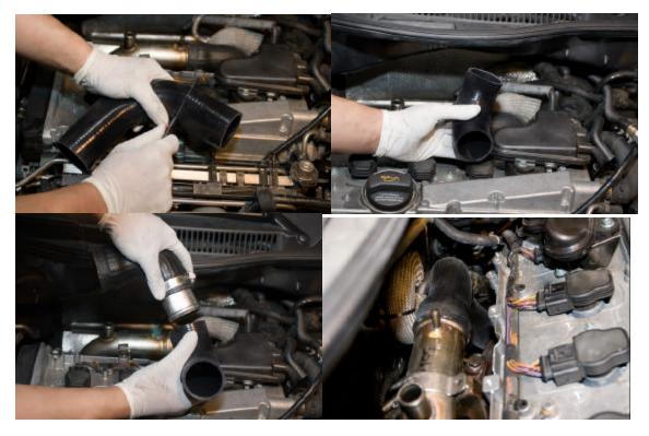
18. Slide pieces together: 2" stainless coupler to stock 90 degree rubber and connect other end of 2" stainless coupler to newly cut short elbow (other end into GT2X turbo). Clamp down all hoses with clamps provided.
