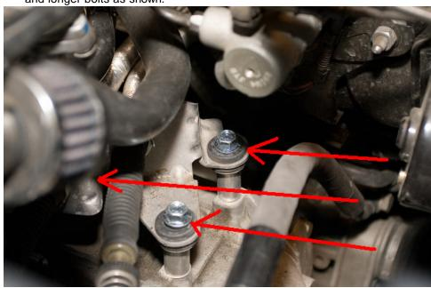
c. Once the shifter bracket is remounted with the spacers, re-install the shifter cable ends into the shifter mechanism and re-install the retaining clips.
