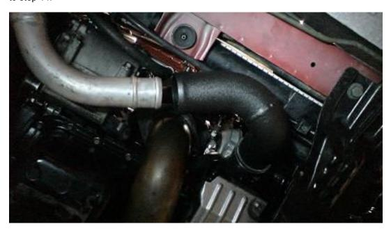
14. Install the 2.5" lower intercooler pipe as shown (join between the compressor discharge pipe and the passenger side of the intercooler).
