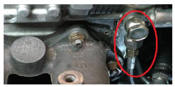
5. Slide rubber end of factory rear coolant hose back into the factory barb and clamp down just like on factory stock turbo.
