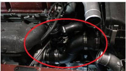
11. Re-install the rubber elbow on the upper intercooler pipe and prepare the radiator hose for reinstall of the radiator.
