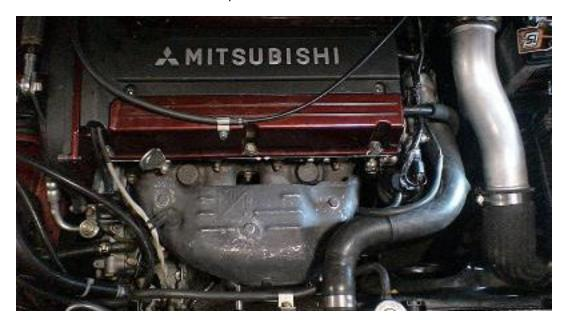
13. Underneath the vehicle. Install the compressor outlet pipe (replaces the stock J-pipe)provided and align to factory lower intercooler pipe.
