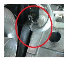
6. Slide the rubber end of the front coolant line assembly (braided line assembly) provided. Slip onto the barb on the waterneck and clamp down as shown in picture.
