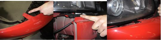
2. Carefully reinsert sides of the bumper cover for proper alignment:
