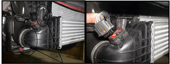
3. Unbolt the (2) bolts holding intercooler to front of radiator at two bolts shown
