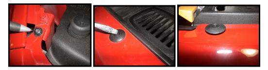
2. Unscrew and remove the (5) screws on the inside of the passenger side fender lining then repeat on the driver side fender lining, behind the bumper cover. Turn the steering wheel to turn wheel/tire as necessary to expose the fender lining. Also, remove lower mounting bolt on each bottom side of the wheel well (as shown on bottom right)
