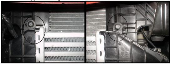
4. Unbolt the MAP sensor from the stock intercooler and slide it into the sensor holder on the ATP intercooler and bolt down using the NEW 4mm bolt provided:
