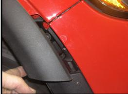
4. Pull away on bumper cover gently and slide off the vehicle as shown:
