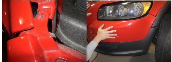
3. Make sure bumper cover is fully re-attached and appear to be in proper alignment with headlights, fenders, fender trims, etc:
