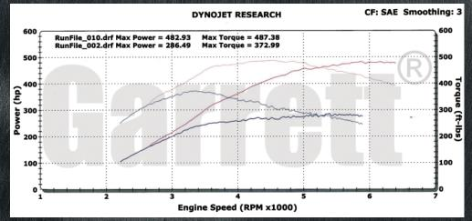
Comparison of Garrett Turbo Kit before and after tuning. Stock Ford Mustang GT horsepower is approximately 230 BHP
