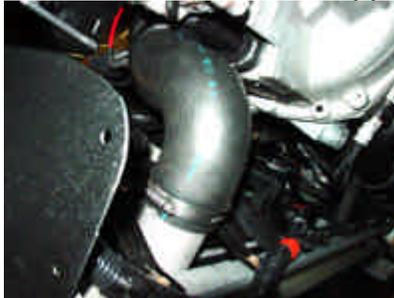
3. Locate stock pressure pipe between throttle body and intercooler and remove by unscrewing 2 hose clamps (1 at t-body and 1 at intercooler). Caution: remove sensor connector and air fitting before remove stock pressure pipe.
