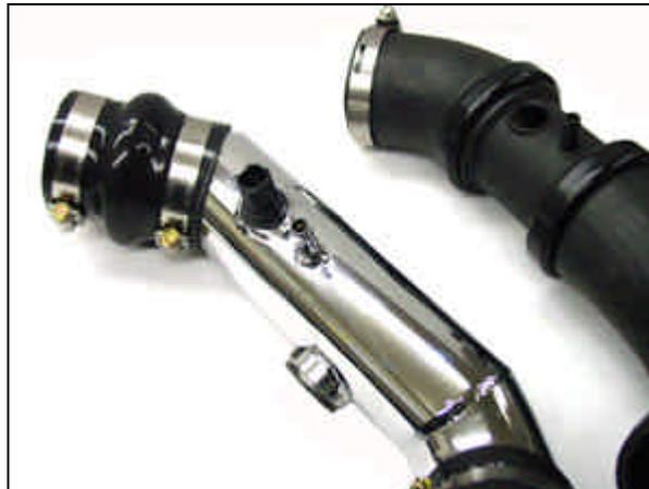
4. Pull air sensor with rubber grommet from stock pipe. Twist sensor and grommet onto new pipe as shown. Moisten grommet with water to make install easier.
