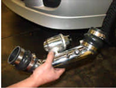
7. Install newly assembled pipe between t-body and intercooler.
