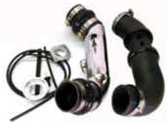
Notice that flanges for different style BOV types are just “hats” that twist onto the threaded fitting on the UPP pipe. Customer specifies BOV type at time of order so that correct top hat is included for the particular BOV the customer is using.
