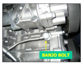
Note: Absent from the above picture is the turbo. This is the banjo bolt at the oil feed port on the engine.
