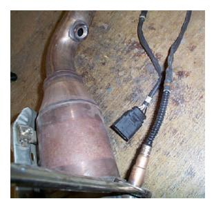
6. Using 22mm wrench, carefully remove 02 sensors from the stock downpipe. Mark the front 02 sensor (larger wire plug) vs. the rear 02 sensor (smaller wire plug) for appropriate reinstall.
