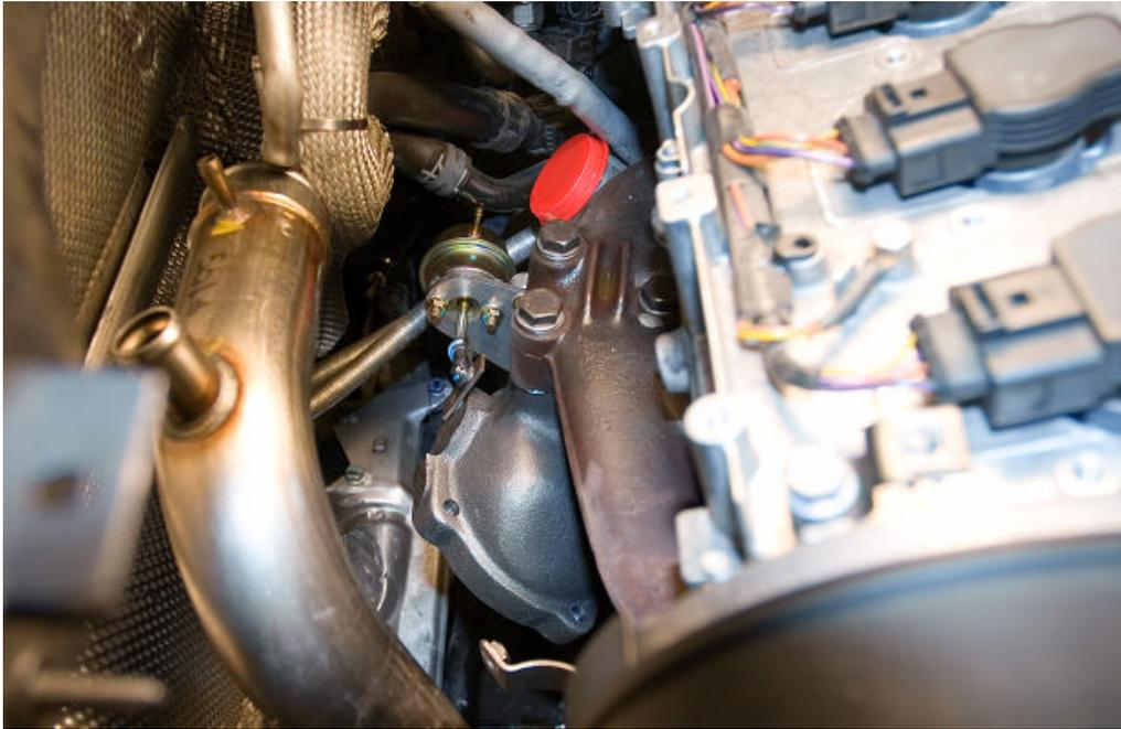
13. Bolt on the new eliminator turbo as shown using new bolts, gaskets, and washers provided.
