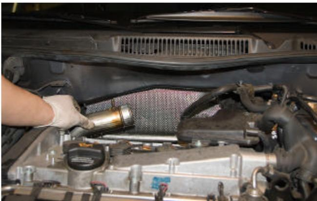
8. Prepare all turbo exhaust parts for removal.
