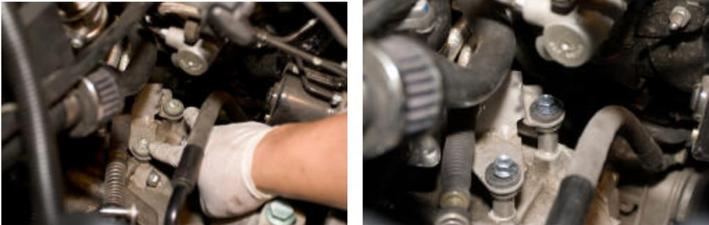
20. Use the Shifter Bracket Spacer Kit to Space bracket 1" higher as shown above.
