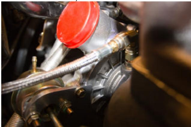
17. Use compressor outlet pieces provided to construct the outlet adapter (to stock compressor outlet hose).
