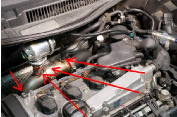
3. Unscrew hose clamp holding diverter valve/BOV to stainless pipe.
