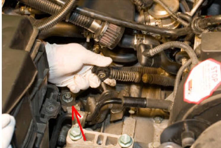
2. When slipping the cable end back on to the shift level, make sure that the lever doesn't get pulled in either direction due to altered cable length.
