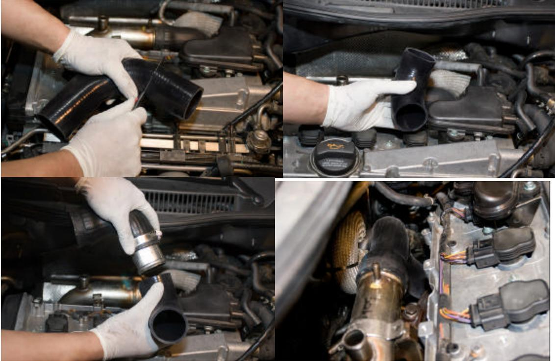
18. Slide pieces together: 2" stainless coupler to stock 90 degree rubber and connect other end of 2" stainless coupler to newly cut short elbow (other end into GT2X turbo). Clamp down all hoses with clamps provided.
