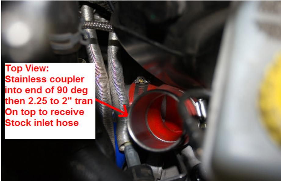
24. With airbox and MAF pipe in original location, run the stock inlet hose into new connection as show:
