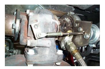
4. Bolt Downpipe to exhaust side of turbo. Top bolts: 8mm x 25mm, bottom bolt 20mm.
