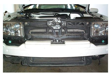
Remove foam and unbolt bumper support bar. 4.
