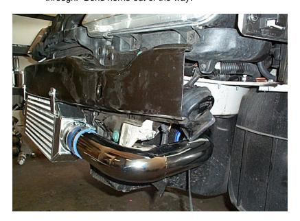
11. Install remaining pipes starting with turbo outlet.
