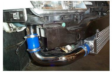
10. Install intercooler outlet pipe. Cut hole through plastic lining to allow pipe to pass through. Bend horns out of the way.
