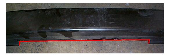
Measure the center point of both the intercooler and bumper support bar. Drill 2 holes 7. and bolt intercooler to the bumper support bar. Top of intercooler must sit flush against the bottom of bumper support bar.
