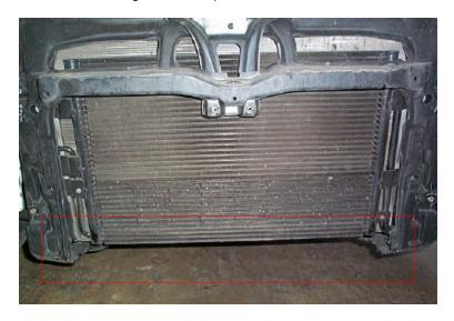
6. Cut away the lower lip on the bumper support bar. This allows the bottom of the intercooler to sit directly above the lip spoiler.
