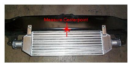
8. Reinstall the bumper support bar with intercooler attached. Insure that the intercooler core sits flush against the front of the A/C condenser (smaller radiator).
